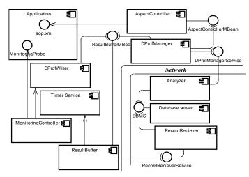
Figure 1. Deployment diagram of the DProf monitoring system
